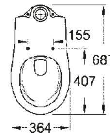
39 429 000 Floorstanding WC for closed coupled combination rimless, vertical outlet
