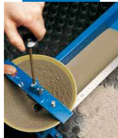
Flow test recording to UNI 13395-2
