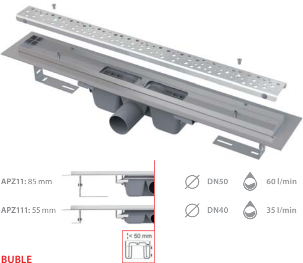
APZ11 Antivandal, APZ111 Antivandal Low Shower drain Antivandal with grid (300, 550, 650, 750, 850, 950, 1050, 1150 mm)
